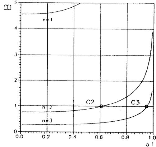
Figure 3: "Breaking-away" point B versus  $a_1$  for  $n=1,2,3$ .
