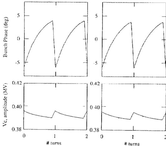
Figure 1. Modulation of the bunch phase and the cavity voltage due to the bunch gap calculated by two different methods; (left) direct calculation in an iterative way and (right) utilizing the transfer function.
