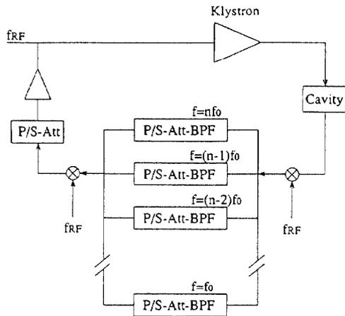
Figure 3. Gap transient compensation system modulating the cavity input power with revolution side bands.
