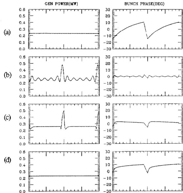
Figure 5. Simulation results of gap transient compensation modulating the rf power; (left) generator power and (right) the bunch phase modulation. From top to bottom is shown; (a) without any modulation of input power, (b) with revolution side bands, (c) with a pulse modulation for the phase and amplitude, and (d) with a pulse modulation only for the phase. The bandwidth of  $\pm 5$  times revolution frequency in (b) and the group delay of 1/3 of the gap width in (c) and (d) is assumed.
