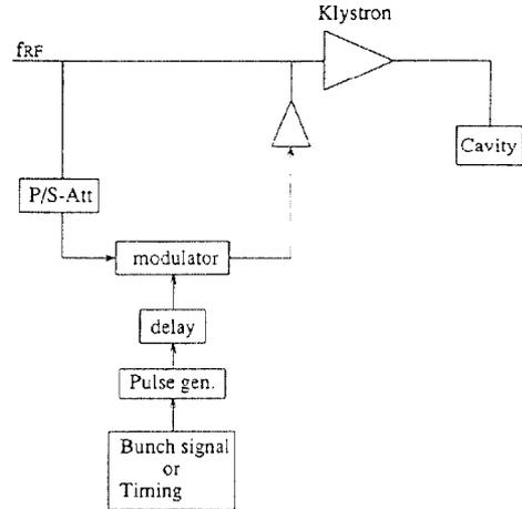
Figure 4. Gap transient compensation system modulating the cavity input power with a pulse corresponding to the gap.
