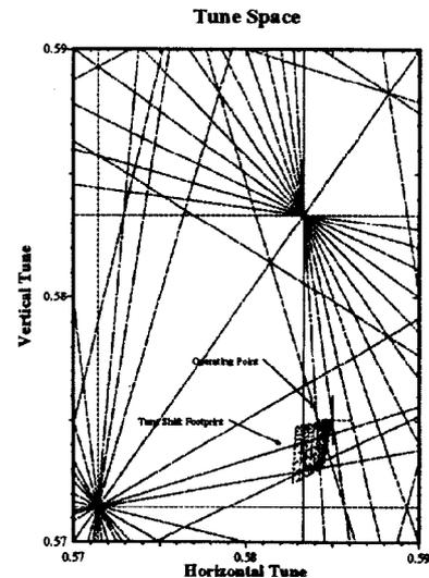
Figure 3: Tune Shift vs. Amplitude for  $\beta^* = 1.7\text{m}$ .
