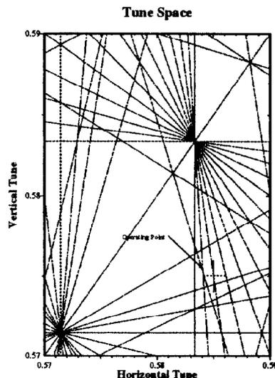
Figure 1: Resonance Diagram Showing the Tevatron Operating Point.
