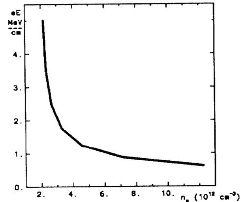
Fig.2. The acceleration rate as a function of the plasma density; beam current density is fixed at  $5 \text{ kA/cm}^2$
