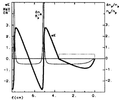
Fig.1. The distributions of the perturbed plasma density,  $\delta n_p/n_p$ , and the longitudinal electric field,  $eE$ , behind electron bunch (the bunch itself is shown with the dotted line); beam and plasma parameters see in the text.
