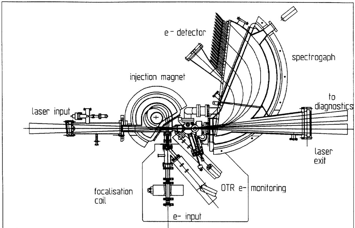
Figure 1: Experimental setup for the beat-wave acceleration
