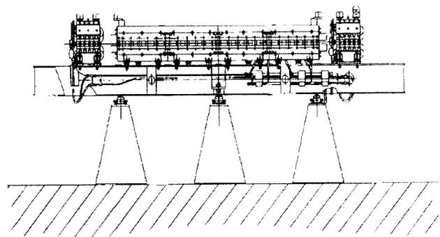
Fig. 2: View of a full synchrotron FODO cell.
