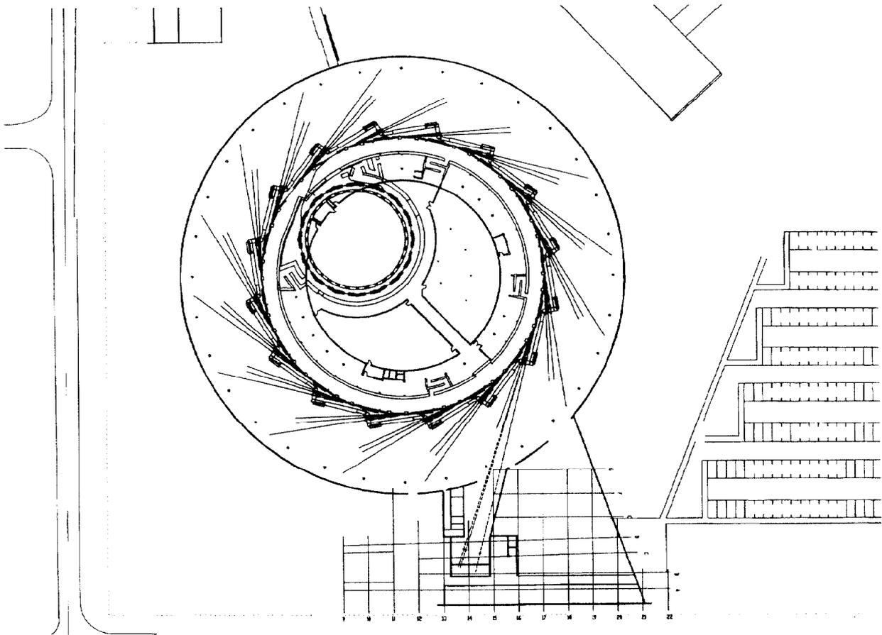
Fig. 3: General layout of the BESSY II experimental hall with storage ring and injectors in the center. SR beamlines are indicated.
