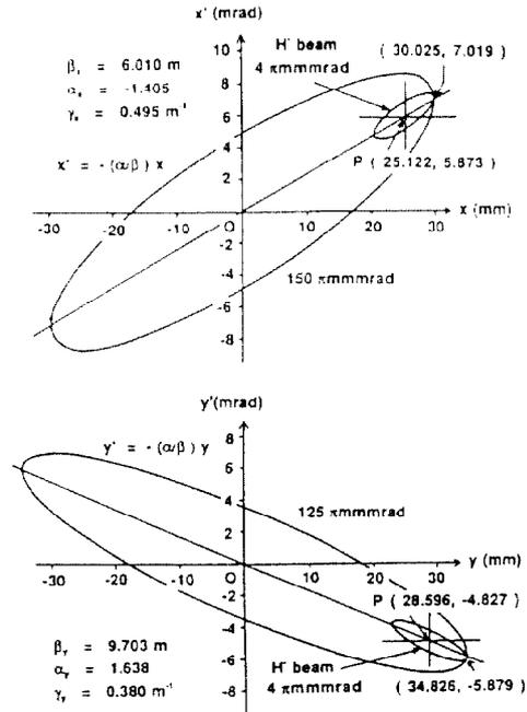
Fig. 4 Emittance ellipses of the injected and ring beam at the injection point
