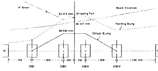
Fig. 6 Offset bump system and the location of the stripping foil for the horizontal plane injection
