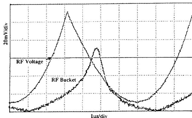
Figure 2: A parabolic RF waveform and the corresponding bunch of the beam measured on a pickup in the ring.
