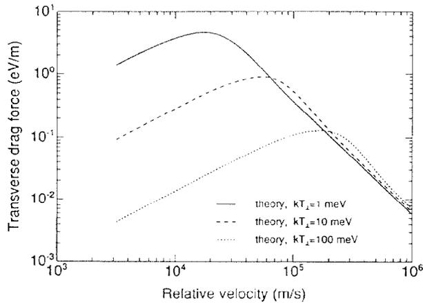
Figure 7: Theoretical transverse cooling force as a function of the relative velocity between ions and electrons.
