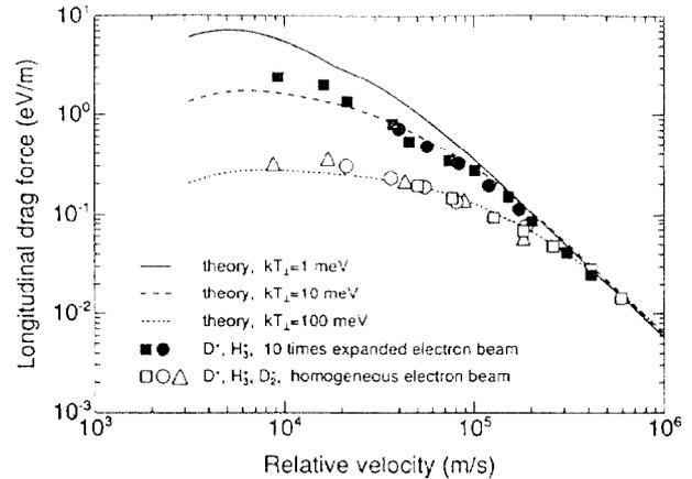
Figure 5: Experimental and theoretical longitudinal drag force as a function of relative velocity between ions and electrons. The theoretical curves are not quite smooth due to the non-analytic expression used for the Coulomb logarithm.
