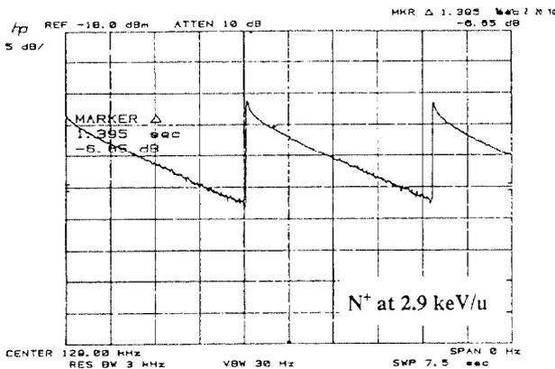
Figure 4: The decay of  $N^+$  ions stored in the ring at 2.9 keV/u
