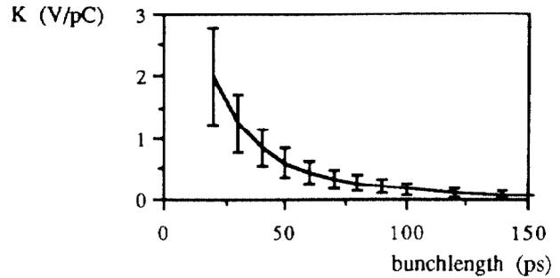
Figure 5 - Parasitic mode loss factor  $K$  of a kicker, calculated as a function of the bunchlength.
