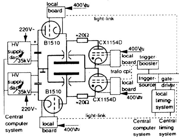
Figure 3 - Schematic layout of the kicker pulsed power supply
