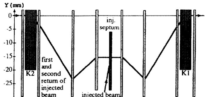
Figure 1 - Schematic layout of the AmPS 3-turn injection process using the kickers (K1,K2) and the injection septum.
