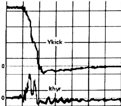
Figure 4 - Measured kicker plate discharge in bench test. Scale is 5 kV/div, 106 A/div and 50 ns/div respectively.
