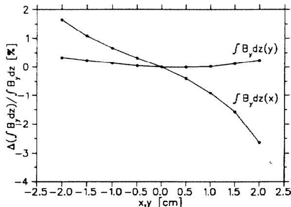
Figure 4. Variation of integrated field in the steerer magnet with transverse position.
