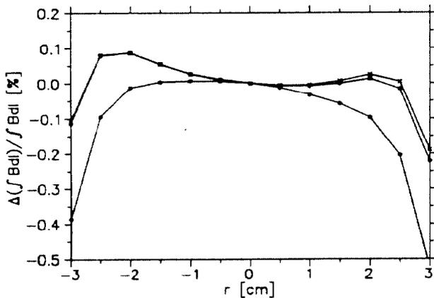
Fig.2. Integrated field uniformity of the 31.4° dipoles at 400 A (upper curve), 605 A and 833 A (lower curve).
