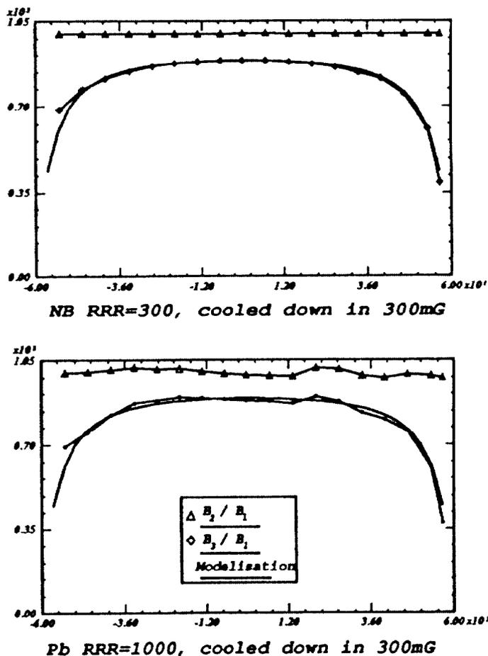
Fig.2: the ratios  $B_2/B_1$  and  $B_3/B_1$  versus the position (mm) on the plate
