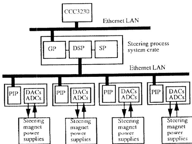
GP: Gateway Processor. DSP: Database Server. SP: Servo Processor.
