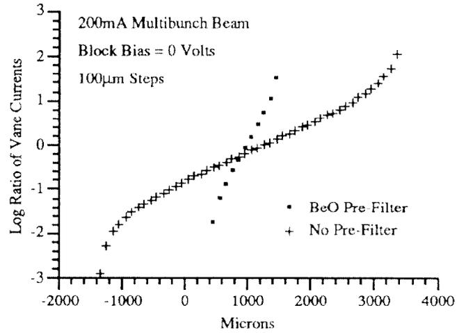
Figure 4. Effect of 0.5 mm BeO Window on TVM Output.
