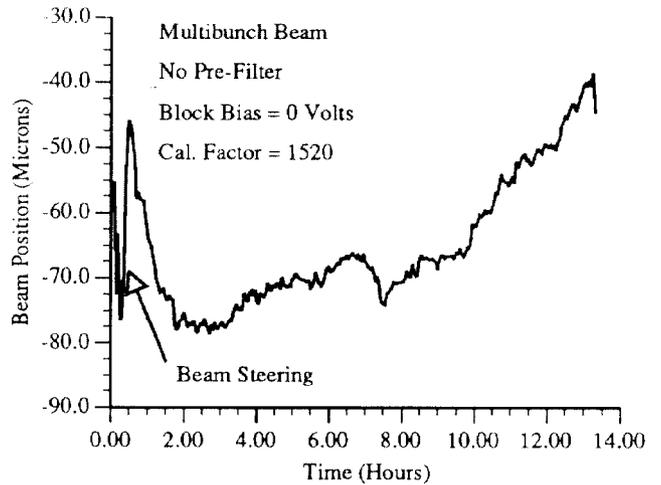
Figure 5. Beam Position Drift 4 m from Source.
