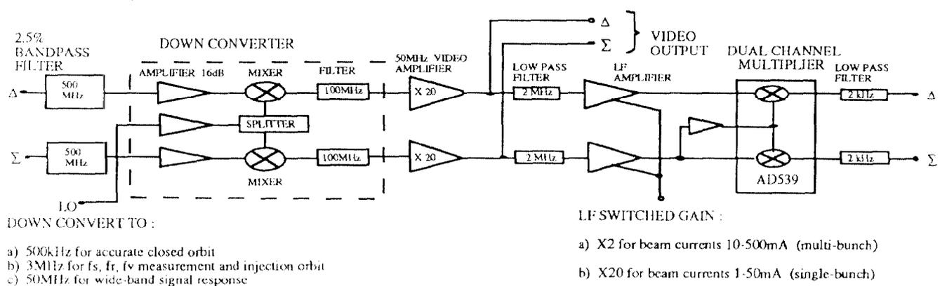
Figure 1. BPM Down Converter and LF Detection System
