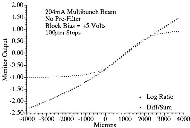
Figure 2. Comparison of  $\Delta\Sigma$  and Log Ratio Outputs.
