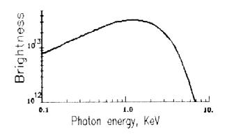
Figure 2. Spectral brightness of the synhrotron radiation from the PSR-2000 dipole magnets.
