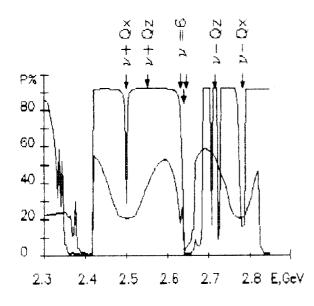
Figure 4. Equilibrium degree of polarization for the PSR-2000 lattice.
