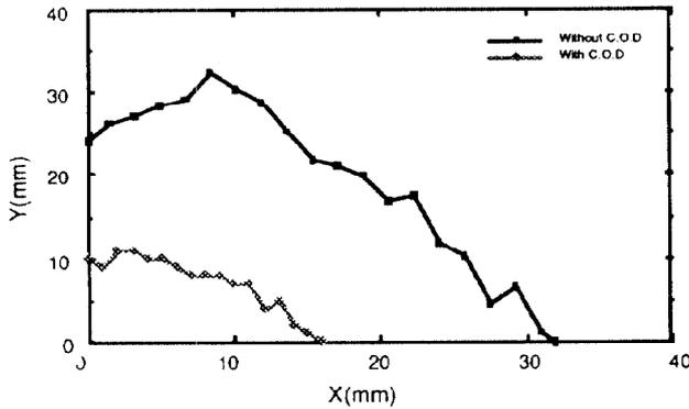
Fig. 1 Dynamic aperture with and without closed orbit distortion.
