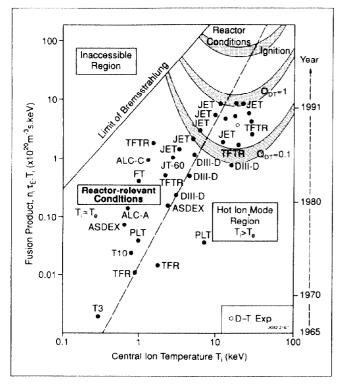
Fig. 3: Overall performance of the fusion product as a function of central ion temperature for a number of tokamaks
