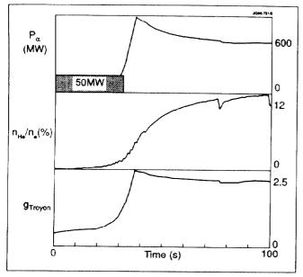
Fig.6: Model of a first reactor plasma using the L-mode transport model tested against JET results
