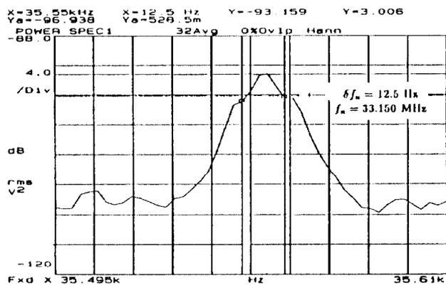
Figure 2: Schottky-spectrum of less than 1000  $\text{Bi}^{82+}$  ions, stored and cooled in ESR at 230 MeV/u, corresponding to  $\delta p/p \approx 6 \times 10^{-7}$ .
