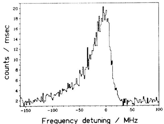
Figure 1: Laser excitation spectrum of a  $\text{Li}^+$  beam at about 2 MeV/u after successive electron and laser cooling at TSR. The 35 MHz-width corresponds to a relative momentum spread (FWHM)  $\delta p/p \approx 10^{-6}$ , i.e. to a longitudinal beam temperature of 200 mK.
