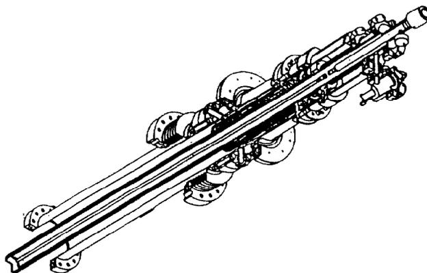
Fig. 4: CERN adjustable power coupler
