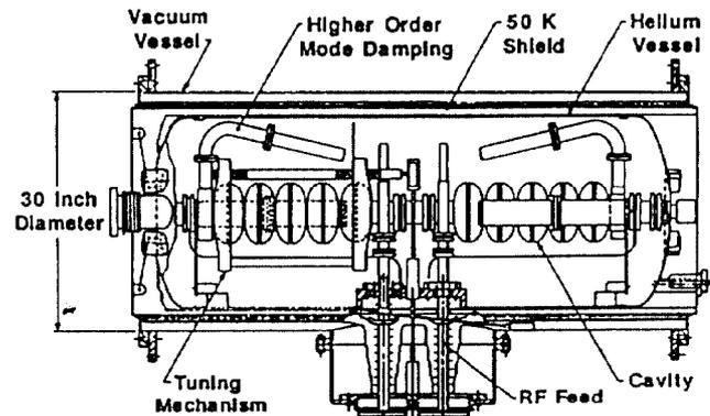
Fig. 3: CEBAF cavity pair with power- and HOM couplers
