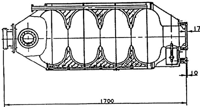
Fig. 2: DESY 4-cell cavity with He-tank and Al-'fillers'
