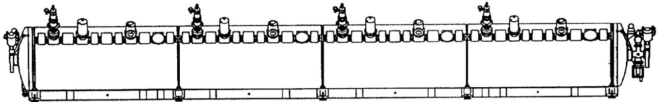
Fig. 6: The CERN 4-cavity module with main coupler and cryogenic domes
