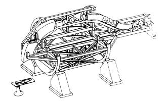
General view of the structure from which one fourth has been removed in order to show clearly the beam line magnets.
