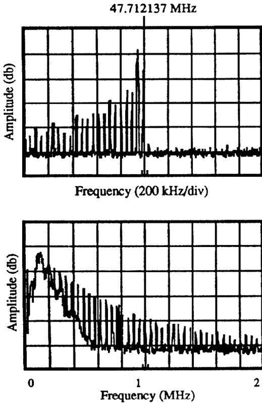
Fig. 1(a) Frequency spectrum near pump frequency  $\Omega_0 = 1000\omega_0$  (b) low frequency spectrum. Lines are spaced by one revolution frequency.
