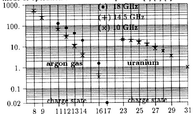
Figure 1: Extracted ion currents ( $\mu\text{A}$ ) from [4] [5] [6]. The same behavior is observed for other elements. These data are somewhat puzzling as the predicted scaling  $\max(I_q) \sim \omega_{rf}^2$  or  $\sim B^2$  is not really observed. This frequency scaling [1] was suggested by the statement that the maximum electron density of the plasma  $n_e$ —and consequently the maximum extracted ion currents, was limited in such a way that
