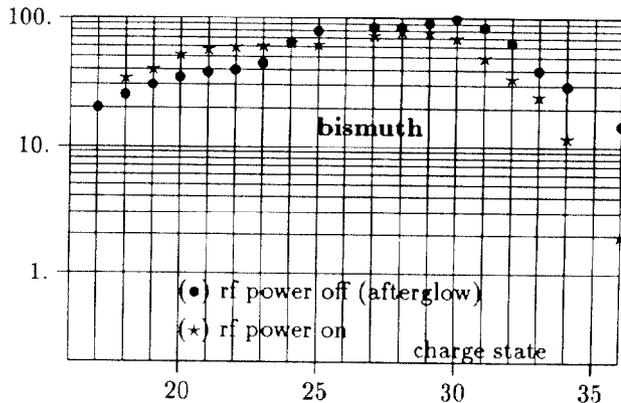
Figure 4: Enhanced ion currents ( $e\mu A$ ) in afterglow from [8]. This phenomenon is interesting of itself to obtain very high ion currents of high charge states  $q$  in short pulses ( $\sim 1$  ms at a few Hz), and is well suited to synchrotron injectors (100  $e\mu A$  of  $Bi^{30+}$  are obtained).
