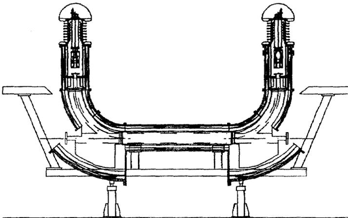
Figure 1: Electron Cooler
