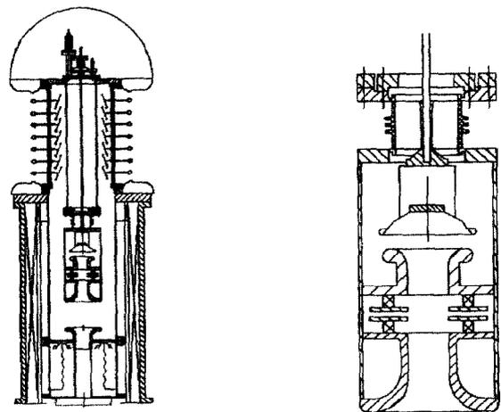
Figure 2: Electron Gun and Acceleration Gap
