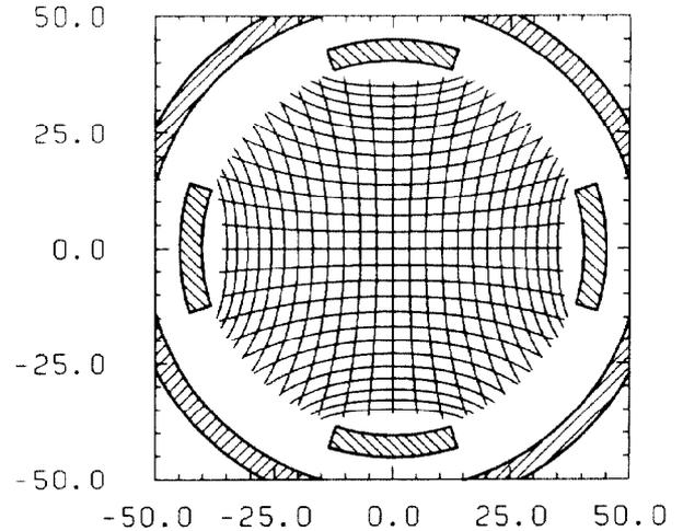
Fig. 6 Lines of equal position sensitivity in 2.5 dB steps as predicted by the wall current model
