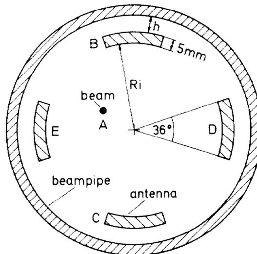
Fig. 1 Cross section through warm pick-ups type Au, In, Hl and Hr
