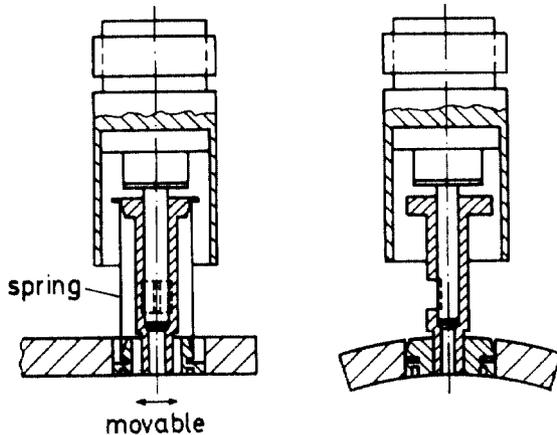
Fig. 3 Scheme of the antenna support
