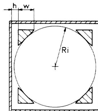
Fig. 2 Cross section through the ZEUS pick-up (type Zr)
