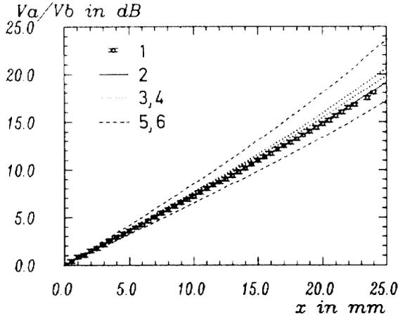
Fig. 5 Position sensitivity of the type Au pick-up along the major axis
