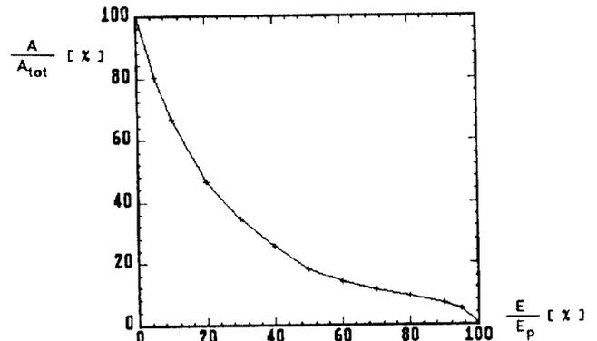
Fig. 5: Relative surface area A/A<sub>tot</sub> of the spherically shaped single-cell cavities at which the normalized electric surface field is greater than E/E<sub>p</sub>. For 3GHz A<sub>tot</sub> is about 218 cm<sup>2</sup>.
