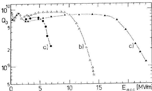
Fig. 3: Q<sub>0</sub>(E<sub>a</sub>) dependence measured for SW1 at 1.6 K initially (a) and after 30 min rf- (b) and 45 min He-processing (c).
