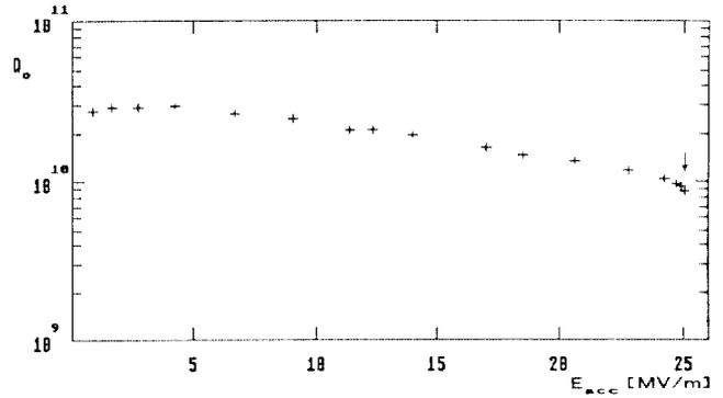
Fig. 4: Q<sub>0</sub>(E<sub>a</sub>) dependence measured on S3 at 1.4 K. The arrow marks the field limitation by quenching
