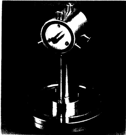
Photo 3 : Beam current transformer of the heavy ion source Dioné
