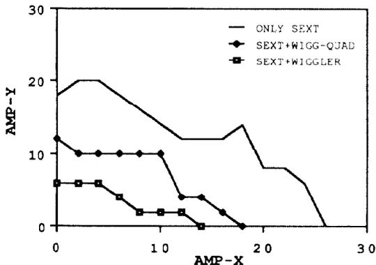
Fig.2. Dynamic aperture with alpha-matching
