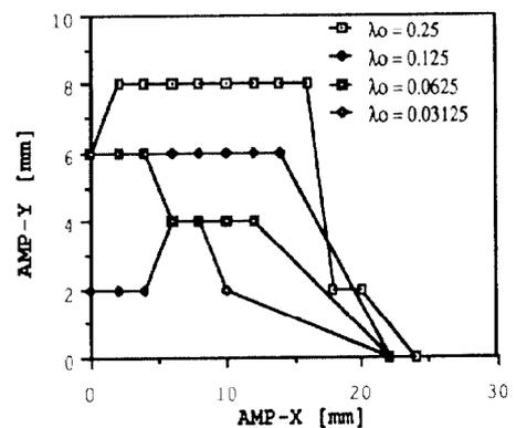
Fig.10 Effects on period length on dynamic aperture
