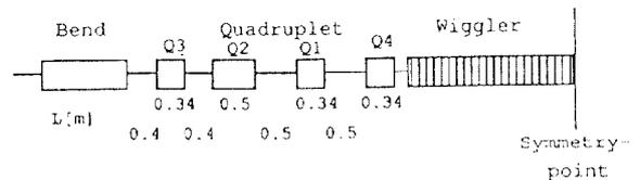
Fig.4. Structure for quadruplet matching
