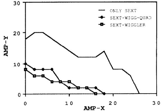
Fig.3. Dynamic aperture with beta-matching
