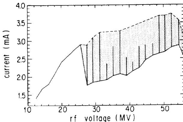
Fig. 1. An example of the inhibit band.  $\nu_x = 36.605$ ,  $\nu_y = 38.730$ ,  $\xi_x = 0.95$ ,  $\xi_y = 0.76$ .
