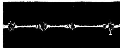
Fig. 2. Beam blow up observed by button electrodes. Horizontal scale is 2msec/div.
