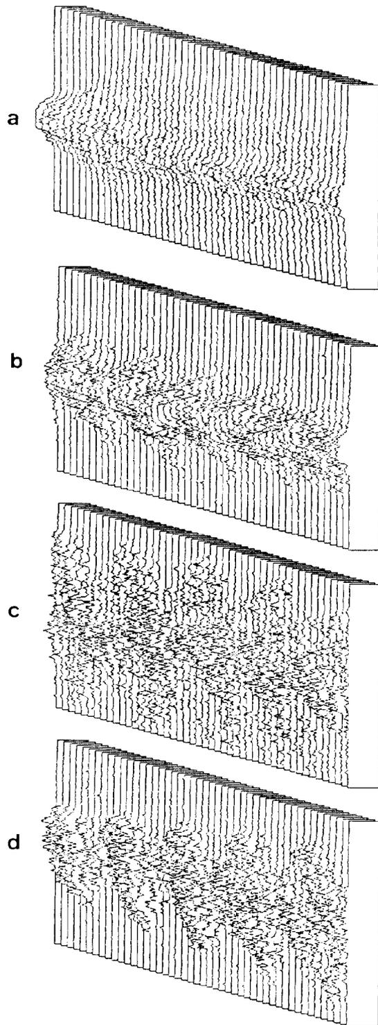
Fig. 4. Computer-processed streak pictures taken at the blowup. Vertical scale is  $1.33\text{nsec}$ . Horizontal full scale is  $9.6\text{msec}$  for (a) and  $0.96\text{msec}$  for (b)-(d). Beam current is (a)  $2.6\text{mA}$ , (b)  $2.7\text{mA}$ , (c)  $2.6\text{mA}$ , and (d)  $2.0\text{mA}$ .
