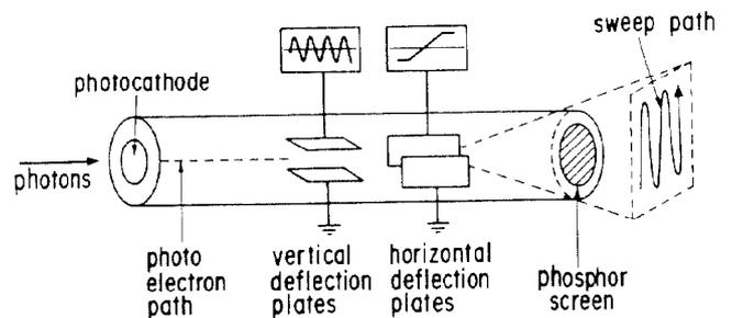
Fig. 3. Principle of the streak camera with dual time base.
