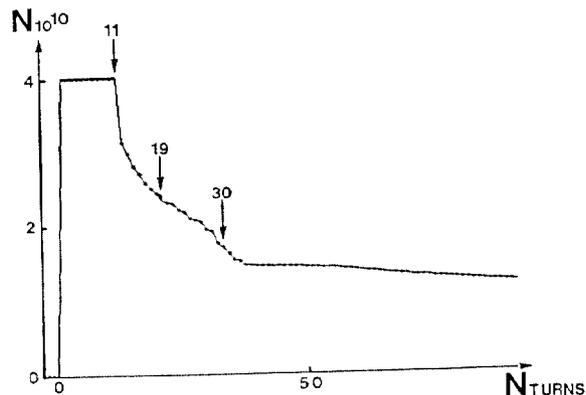
Fig. 1 : Beam loss after injection as a function of the number of turns
