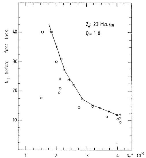
Fig. 3 : Number of turns before beam loss as a function of bunch intensity
