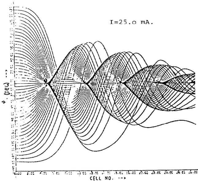
Fig.4: Adiabatic bunching of beam in RFQE .
