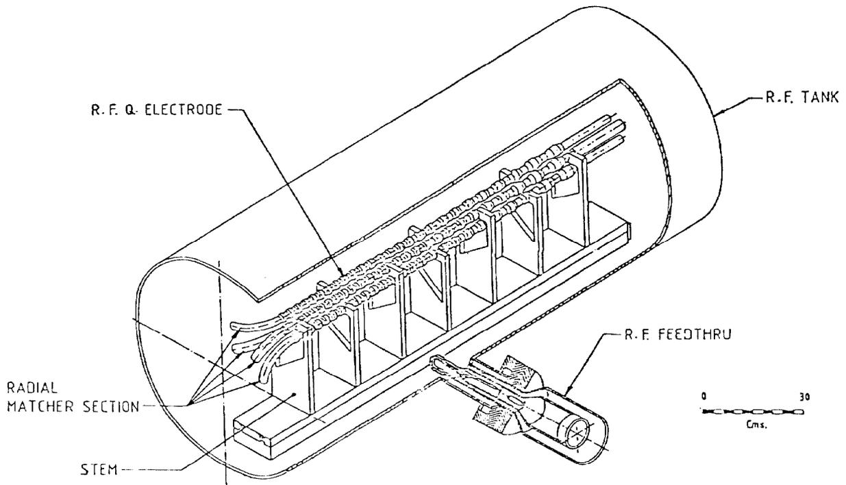
Fig.6: Assembly of RFQE
