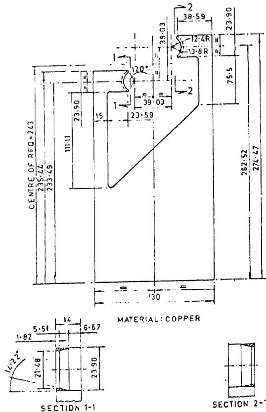
Fig.7: The details of one of the Stem.
