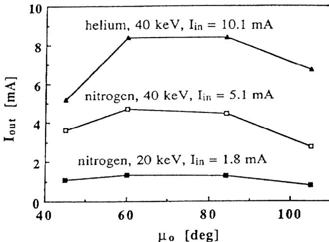
Fig. 2. The ion current transported through the LEBT section as a function of the zero current phase advance per cell ( $\mu_0$ ).
