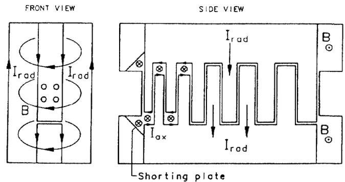
Fig. 3. Accelerating structure. The magnetic field lines surround the accelerating structure, leading to radial currents. Shorting plates force the field lines through the free area, leading to additional axial currents.
