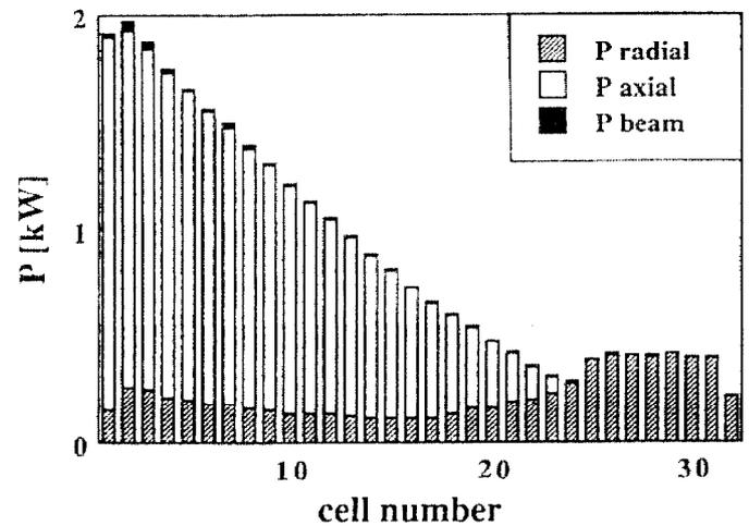
Fig. 5. The estimated distribution of the power dissipation  $P$  along the axis in the accelerating structure of the final design of the resonator cavity.
