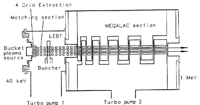
Fig. 1. Set-up of the FOM-MEQALAC experiment.
