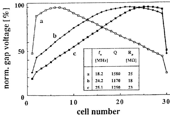
Fig. 4. The measured voltage distribution, normalized to the maximum gap voltage, along the RF-gaps for different structures: (a) conventional set-up, (b) with shorting plates and (c) tuned to the final resonance frequency by a reduction of the gap capacitance at the entrance.
