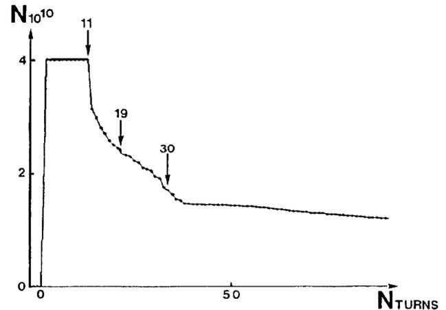
Fig. 5 Positron bunch intensity as a function of the turn number
