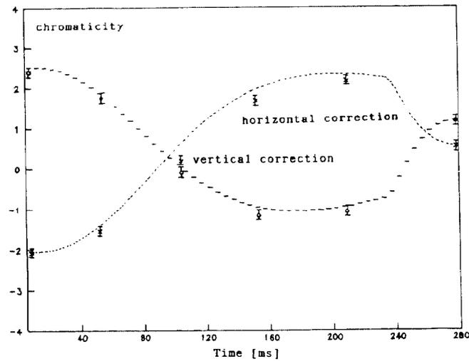
Fig. 3 Applied chromaticity correction along the ramp for a lepton cycle.
