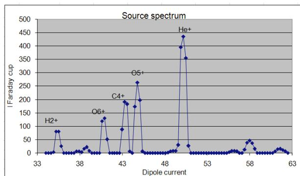
Figure 6: Spectrum of the carbon source. 200  $\mu A$  of  $C^{4+}$  are produced
