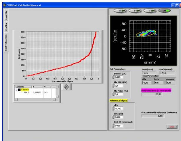
Figure 7: Emittance of the  $C^{4+}$  beam. The total current was 220  $\mu A$
