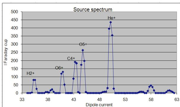
Figure 6: Spectrum of the carbon source. 200 μA of C<sup>4+</sup> are produced
