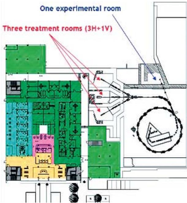
Figure 2: Floor -1 (accelerator level) at CNAO.
