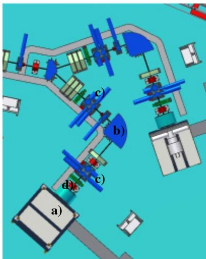
Figure 5: The initial part of the LEBT is used to analyse the beam and comprises: a) source, b) spectrometer, c) diagnostic tanks and d) solenoid.
