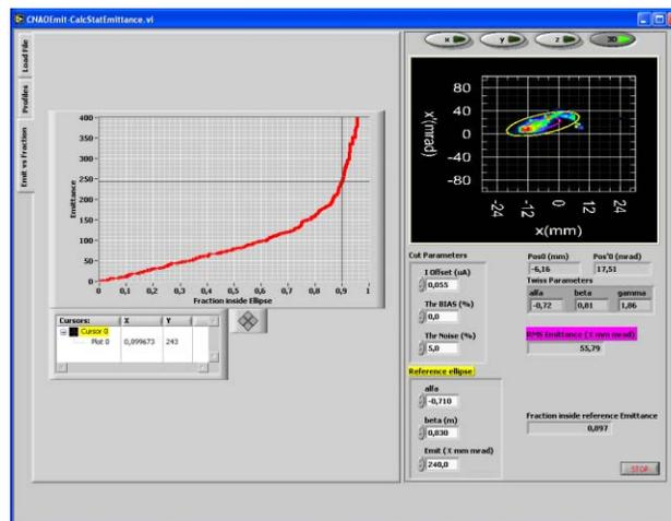
Figure 7: Emittance of the C<sup>4+</sup> beam. The total current was 220 μA
