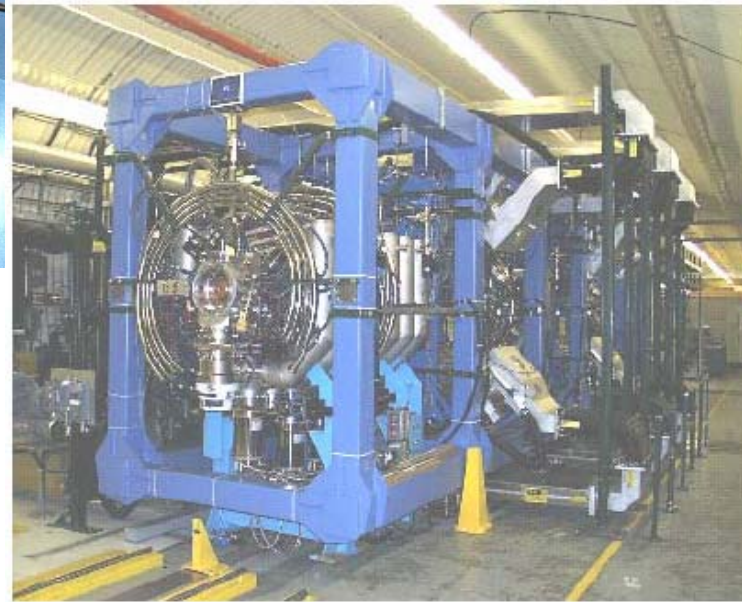
LEDA Radio-Frequency Quadrupole (RFQ) accelerator with injector rolled back
