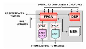
Figure 2: General DLLRF board with DSP and FPGA.
