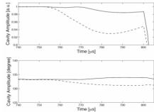
Figure 5: SNS DTL4 cavity amplitude/phase under beam loading with (solid line) and without (dashed) AFF [45].
