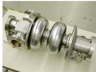
Figure 5: Prototype injector cavity for Cornell ERL 5 cavities of this type are needed.
