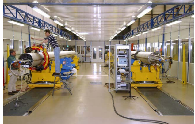
Figure 3: Closure and geometrical verification of the quadrupoles are performed on two alignment benches.
