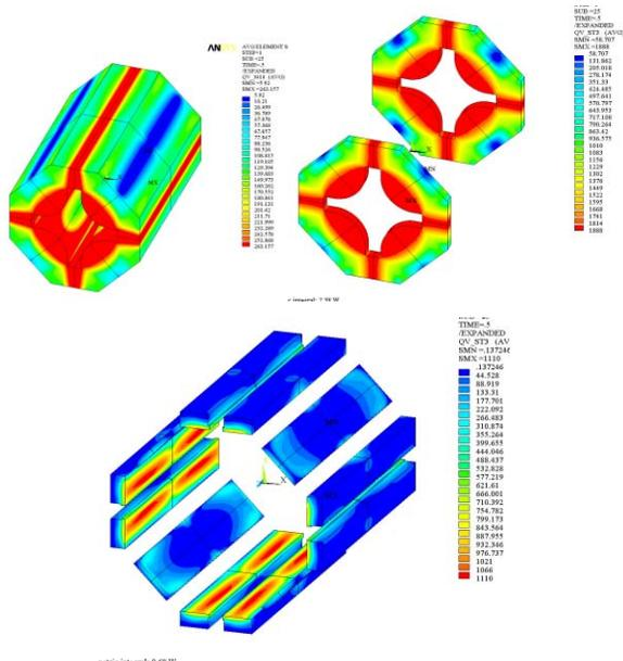
Figure 3: Distribution of hysteresis losses in the yoke, endplates and brackets.
