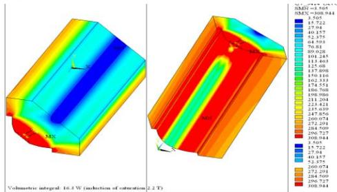
Figure 7: Hysteresis loss distribution in the yoke.
