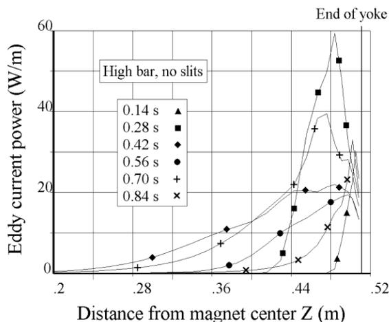
Figure 5: Eddy current loss in the optimized model quadrupole.
