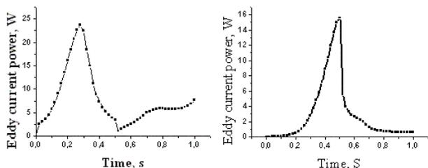
Figure 2: Power vs time in end plates (left) and brackets made from low carbon steel.
