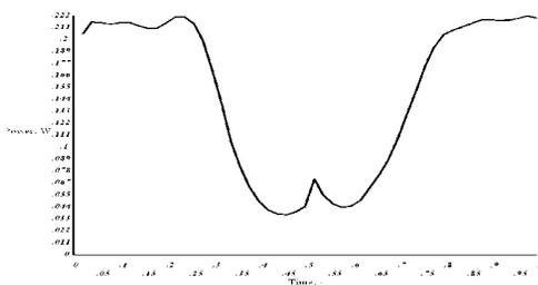
Figure 10: Eddy current loss in the end plates.
