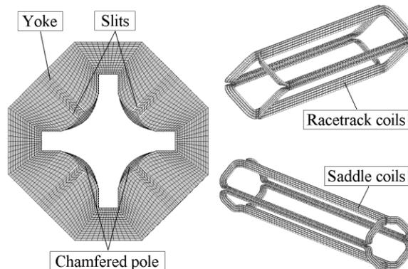
Figure 4: Design of the optimized model quadrupoles.
