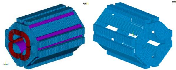
Figure 1: Short ANSYS model of the SIS100 test quadrupole with high bedstead coil end parts and restrain elements (endplates and brackets) separately.
