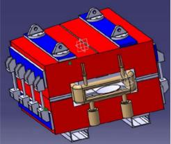
Figure 4: Preliminary design of a CR/Super-FRS dipole, made by the Institute of Modern Physics (IMP), Lanzhou, China.
