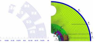
Figure 3: 2D coil design (left) and FEM model for mechanical analysis of SIS300 dipole (right). 1-coil, 2-inter-turn spacers (wedges), 3-key, 4-collars, 5-yoke, 6-outer cylinder.
