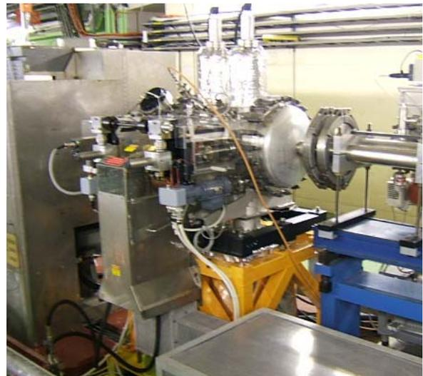
Figure 5: PS ion injection septum P1.SMH26 installed in the ring.
