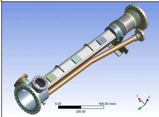
Figure 3: 3D Catia rendering of the vacuum chamber.
