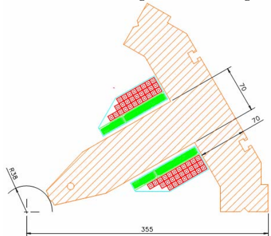
Figure 7: Sextupole cross section.
