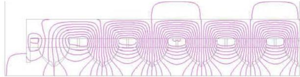
Figure 3: Magnetic lines for  $\sim 1/4, 1/2, 1$  tapering.
