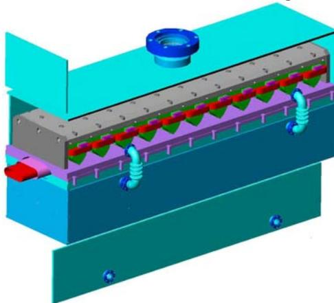
Figure 6: Cold mass view. Two upper side walls opened.
