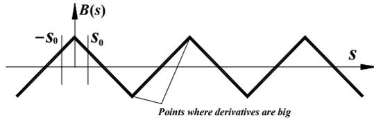
Figure 2: Longitudinal profile of magnetic field with linear dependence between extremes.
