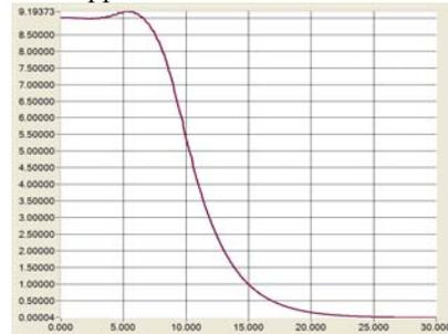
Figure 4: Vertical field across the regular pole in median plane.
