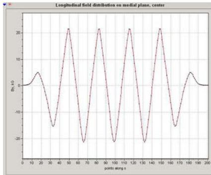
Figure 5: Longitudinal field, kG, dependence (as function of  $s$ ) at  $x=0$  calculated for the wiggler in Fig. 3 with tapering  $\sim 1/4, 3/4, 1$ . Right point on this picture corresponds to  $s=150$  cm.
