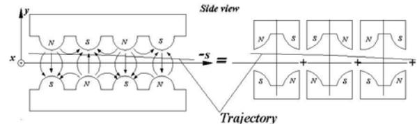
Figure 1: Representation of wiggler as series of quadrupoles with *transverse* orientation.
