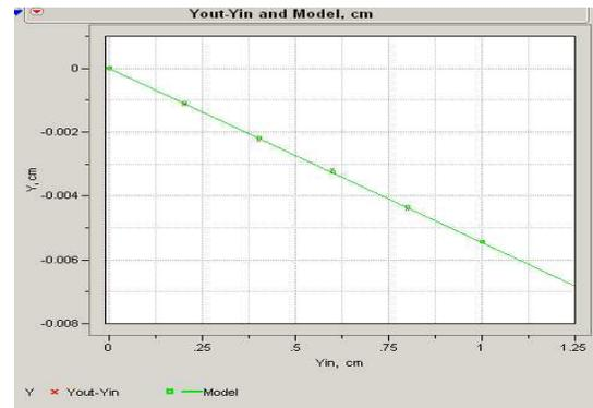
Figure 8: Difference between exit and entrance  $y$  – coordinates and the linear model fit.
