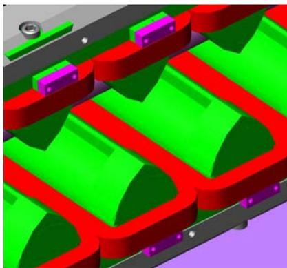
Figure 7: Wiggler cold mass fragment magnified.
