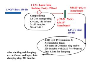
Figure 1: Schematic view of CLIC Compton source.
