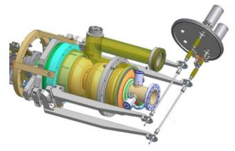
Figure 5: Dual tuning system of the cavity.
