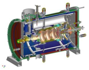
Figure 1: 3-D view of the SRF gun cryomodule.
