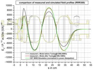
Figure 4: Measured field profiles of the  $\pi$  mode of the RRR 300 cavity before and after tuning.
