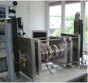
Figure 3: Field profile measuring (bead pull) and warm tuning machine.
