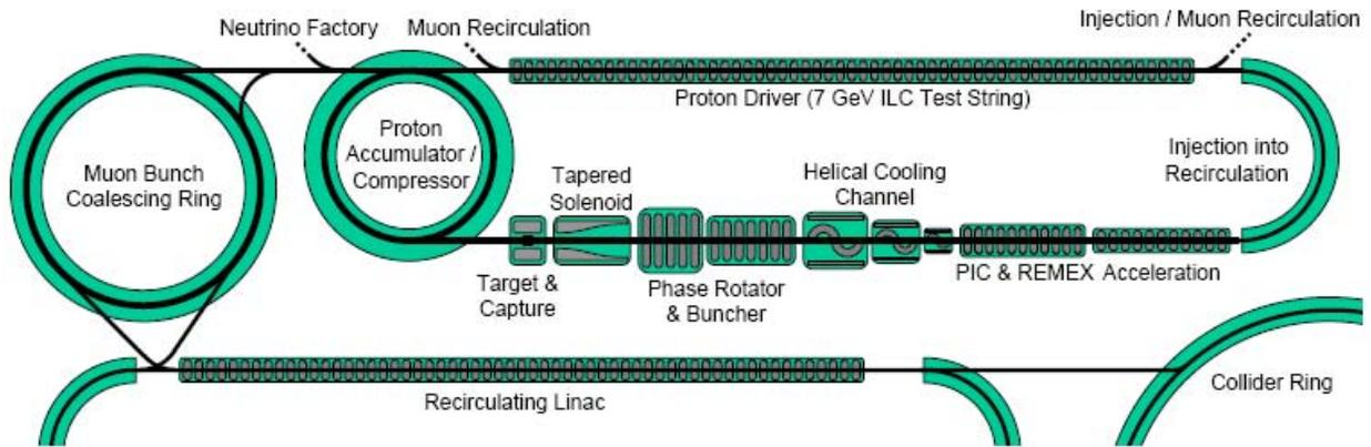
Figure 1: This figure depicts a possible scenario for a muon collider involving a multi-purpose proton driver, extreme muon beam cooling, muon recirculation in the proton driver, bunch coalescing, and synergy with ILC technology.
