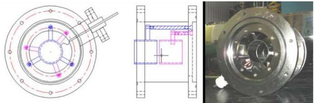
Figure 4: Drawing and photograph of Einzel lens.
