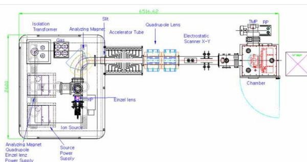
Figure 1: Schematic of 300kV heavy ion implanter.
