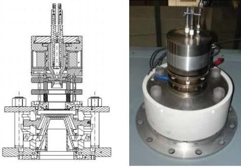
Figure 2: Drawing and photograph of ion source.
