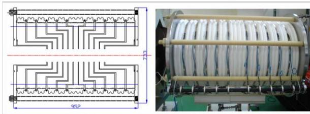
Figure 7: Drawing and photograph of Acceleration tube.
