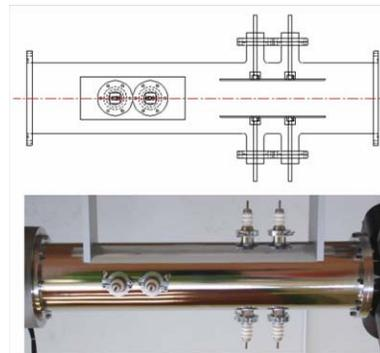
Figure 9: Drawing and photograph of electrostatic scanner.
