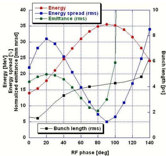
Figure 4: Beam characteristics as a function of X-band rf phase
