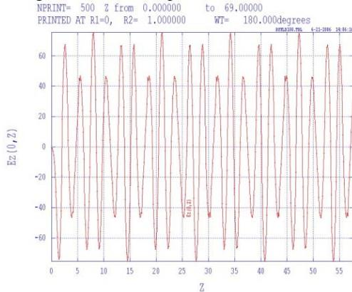
Figure 3: Electric fields of X-band linac
