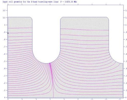
Figure 2: X-band input cell and first cell
