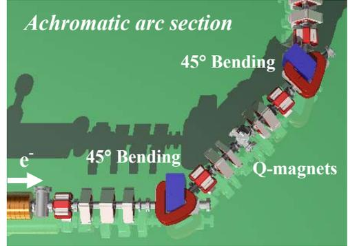
Figure 6: Top view of achromatic arc section
