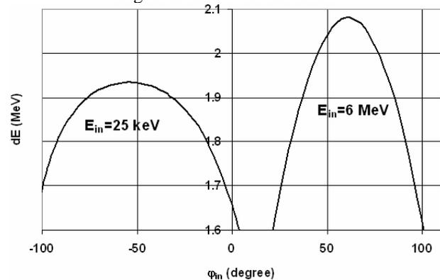
Figure 3: Linac energy gain.
