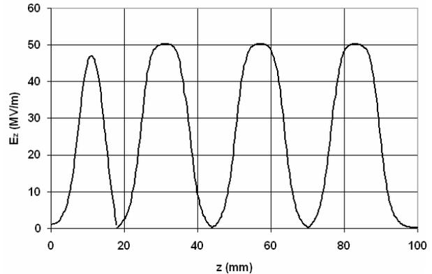
Figure 2: Linac on-axis field.
