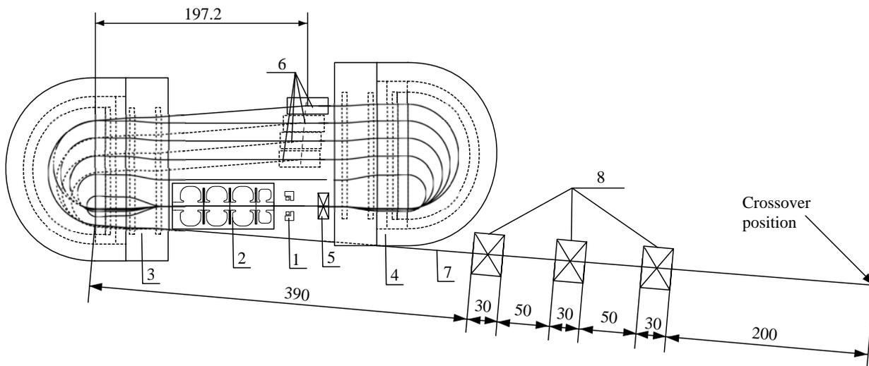
Figure 1: RTM Schematic (dimensions in mm).
