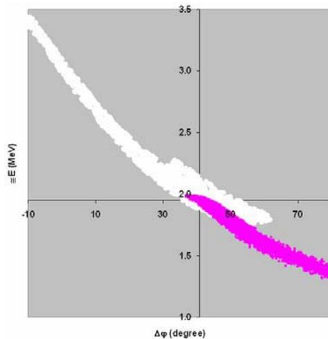
Figure 5: Longitudinal RTM acceptance (white region) and beam emittance (pink region) at 2 MeV.
