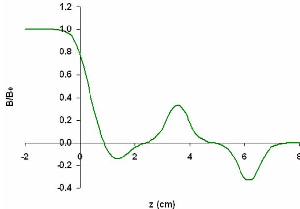
Figure 4: Fringe field of end magnets.
