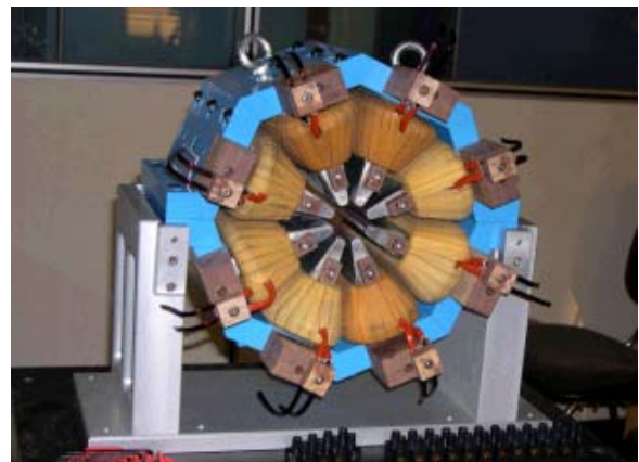
Figure 7: One of the two octupoles to be installed on the TOP linac injector line.
