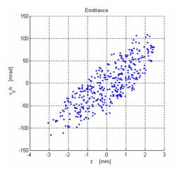
Figure 3: Beam axial emittance at the exit of the inflector.
