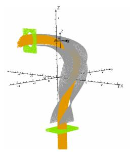
Figure 2: Layout of the spiral inflector crossed by the beam. The electrodes surface are in grey, the collimators are in green and the beam particles in orange.
