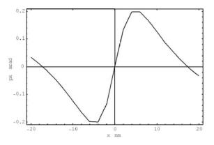
Figure 1: Angular deflection at the exit of the MEPU device operating in linear vertical polarization mode, based on particles with initial location (x,y=0). Tracking was performed using Radia [8] and independently verified using using Cosy [9].
