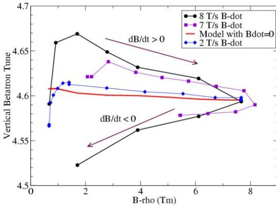
Figure 4: Measured Vertical Betatron Tune vs Magnetic rigidity for 3 different  $\dot{B}$ .
