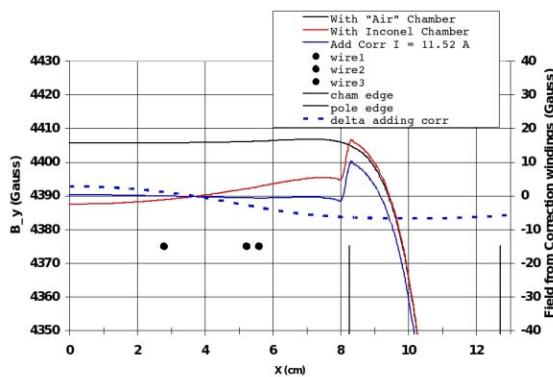
Figure 2: Field on HMP without vacuum chamber, with vacuum chamber, and with correction coils.
