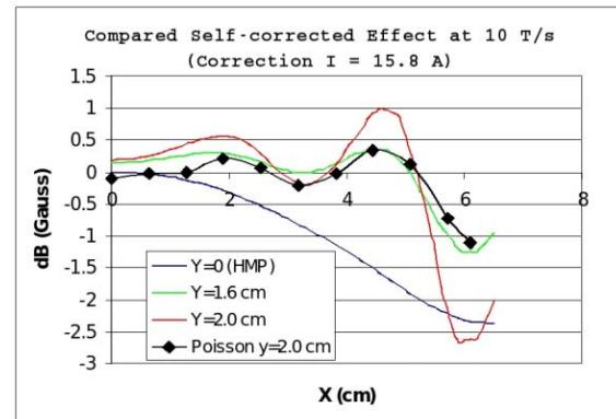
Figure 3: Field distortion for 10 T/s at 0, 1.6, and 2 cm above the HMP with the effect of the correction coils included.
