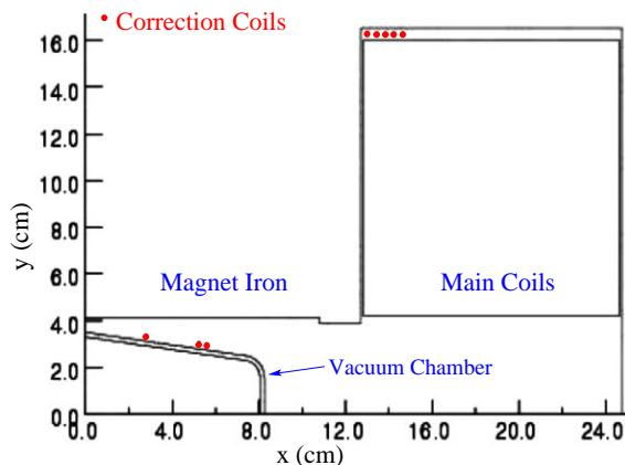
Figure 1: Booster Dipole cross section model used to study eddy currents.
