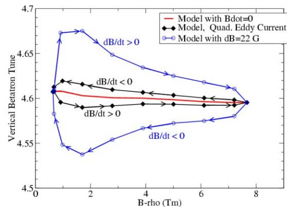
Figure 5: Results for  $\dot{B} = 8\text{T/s}$  of 2 different simulations.
